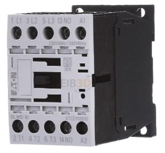
Power contactor 1NO 5.5KW/400V,AC DILM12-10 (230V50HZ) - Magnet contactor 12A 230VAC 0VDC DILM12-...
