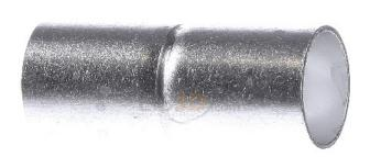
Aluminum push-fit socket AMS-E 20 Material metal, material quality aluminium, surface untreated, quality of the surface coating uncoated, halogen-free, plug-in version, for nominal pipe diameter 20mm, color natural, material of the seal without seal, AMS-E is an aluminum push-fit socket made of extruded Aluminum. This sleeve is used to connect the aluminum tube Alu Steck-ES. VDE 0605 DIN EN 61386-21
