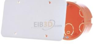
Junction box 47mm 9062-21 Installation type hollow wall, round shape, junction box/box design, single version, connectable, equipment without, diameter 68mm, depth 47 ... 47mm, screw fastening of the devices, housing lead-through through knockout opening, for pipe diameter 20 mm, entry from the rear, number of grommets supplied 0, material plastic, color orange, degree of protection (IP) IP3X, design cover without, screwed cover attachment, functional integrity without, max
