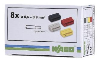
Junction box terminal dgr 8x0.6-0.8mm 243-208 number of terminal points 8, cable diameter 0.6 ... 0.8mm, color dark gray, rated voltage 100V, rated current 6A, suitable for solid conductors, AWG range 22 ... 20, MICRO junction box terminal for solid conductors Ø 0.8 mm 8 conductors Housing color dark gray Cover color light gray Ambient temperature max. 60°C
