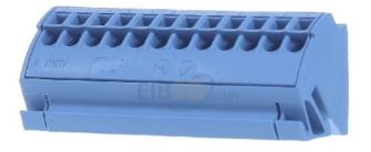
Busbar block 4qmm blue 812-104 Busbar thickness 3 ... 3mm, busbar width 10 ... 10mm, suitable for flat bars, width of the terminal 75mm, max. conductor cross-section 4mm², max. rated operational current le 96A, suitable for round conductor connection, connection block for busbars 10 x 3 12-pin without push button 4 mm²
