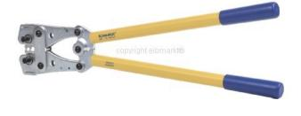
Crimping pliers K 09 Suitable for cable lugs and connectors, hexagonal crimp shape, cross-section 25...150mm², length 650mm, mechanical design/actuation, number of inserts supplied 1, power-saving and low-maintenance mechanical drive. With rotatable profile discs. Exact cross-section assignment through permanent marking on the profile discs. For tubular cable lugs and connectors, standard version.
