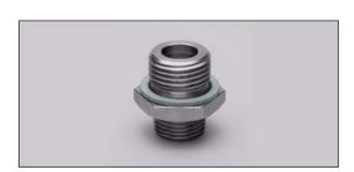
Adapter M18x1.5/G 1/2 E40096, type of accessory=thread adapter, accessories, adapter, M18 x 1.5 - G , process connection: G , immersion depth of the sensor from SID, SFD, TN: , 21 mm, material Housing: V4A (1.4404)
