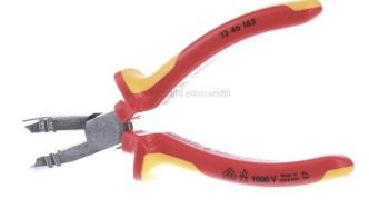
Length 165 mm, Stripping area cross section 0.75..2.5 mm², Stripping area diameter 8..13 mm, Stripping length adjustable no, Notch depth adjustable no, Longitudinal section no, Round cut yes, Spiral cut no, With wire cutter no, Isolated yes, Protective insulation 1000 V yes, Handle version 2 components, ESD tested no, With impact protection no, VDE tested yes
