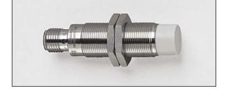
Sensor inductive M18x1 AS-i IGC235, housing design = cylinder, thread, inductive sensors, inductive sensor, M18 x 1, metal thread, switching distance: 12 mm, non-flush mountable, 2-wire, AS-i, operating voltage: 26.5... 31.6 V DC (AS-i), current consumption: 30 mA, plug connection, M12 plug connection, gold-plated contacts, housing material: threaded sleeve: V4A (316L) active surface: LCP colorless fastening nuts: brass
