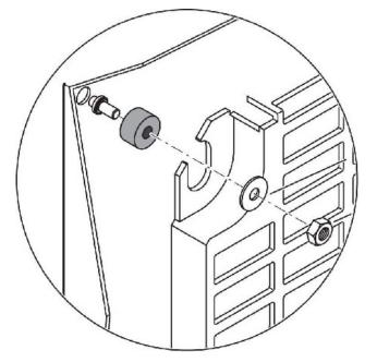
Telequick panel 600x400 - Mounting plate for distribution board NSYMR64
