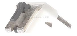
Connection bracket ZV-L2/L3-80A-10 Rated current In 80A, other design, length 35mm, width 15mm, height 12mm, silver-plated surface, plug-in busbar for PLS., CLS., PKN., PFIM, PFHM, (with auxiliary switch), any Switchgear combinations with or without auxiliary switches possible, only a few components, 2 bracket types per rail cross-section for three-phase busbars, common cover profile with end caps for ZV-SS-80A, short-circuit and insulation resistance tested according to IEC/EN 60439-1
