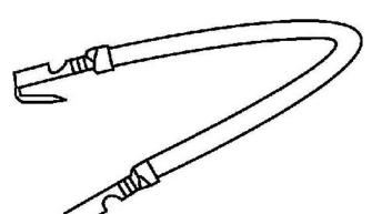
Ground wire L=300mm receptacle - Round wire 4mm<sup>2</sup> L 4182 gn/ge
