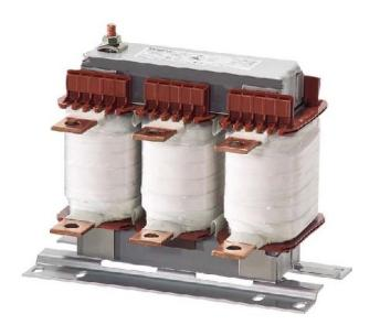
Commutation reactor for power converters - Coil for low-voltage 3-pole 40,5A 400V 4EP3801-6DS00
