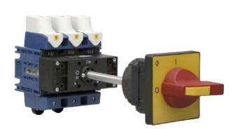
Number of poles=3, With zero (off) position=yes, Rated permanent current lu=63 A, Rated operation power at AC-3, 400 V=18,5 kW, Degree of protection (IP), front side=IP40
