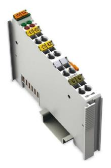
Analog input terminal 2-channel 0-20mA diff. - Fieldbus analogue module 2 In / 0 Out 750-480
