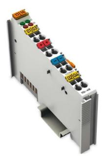
Digital input terminal 2-channel DC24V 3.0ms - Fieldbus digital module 2 In / 0 Out 750-418
