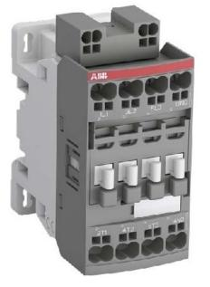
Contactor 12-20VDC/3-pole - Magnet contactor 9A 100...250VAC AF09Z-30-01K-20
