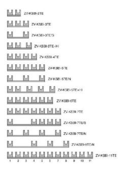
Phase bar 4Ph, 16qmm, fork, 9TE - Phase busbar 1-p 16mm<sup>2</sup> 160mm ZV-KSBI-9TE/N
