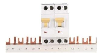
Number of phases 2, Number of poles 1, Pitch 0 mm, Cross-section 10 mm², Length 1000 mm, Width in division units 1, Rated continuous current lu 50 A, Execution of the electrical connection Pen, Isolated yes, Rated surge voltage 4 kV, Conditional rated short-circuit current lq 0 kA, Max. Rated operating voltage Ue 415 V, Rated short-time withstand current lcw 0 kA, Suitable for devices with neutral conductor no, Suitable for devices with auxiliary switch no
