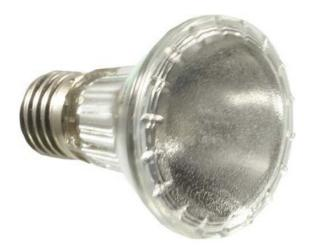
Halogen bulb PAR20 63x82mm E27 220-230V100Wspot - MV halogen reflector lamp 100W 100W 25° 12906
