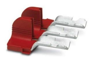
Insertion bridge EB 3-31/PT number of bridged terminals 3, rated current In 232A, isolated, pitch 31mm, color red, insertion bridge, pitch: 31mm, length: 78.4mm, width: 85.7mm, number of positions: 3, Red color
