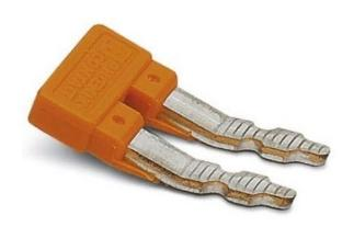
Insertion bridge EB 2- 8 OG Other version, number of bridged terminals 2, color orange, insertion bridge, 2-pole, fully insulated, color of the insulating material: orange
