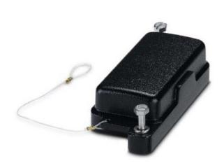
Protective cover B6 Height: 32mm HC-HPR-B06-BCLWH-EBK Shape rectangular, flammability class of the insulating material according to UL 94 other, protective cover B6, with screw locking, material: die-cast aluminum, material protective cover: Al, height: 32 mm, for increased environmental and EMC requirements
