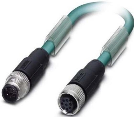
Bus system cable SAC-8P-M12MS1554021 Sheath color other, perm. External cable temperature after installation without vibration -25 ... -25°C, Other category, bus system cable, Ethernet CAT5 (1 GBit/s), 8-pin, PUR halogen-free, water blue RAL 5021, shielded, straight connector M12, A- coded, on straight M12 socket, A-coded, cable length: 5 m
