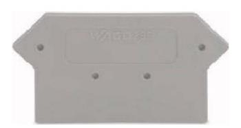
End/partition plate for terminal block Type of end plate, Type of partition, Colour Grey, Thickness 2,5mm, Snap in, Inflammability class of insulation material acc. with UL94 V0
