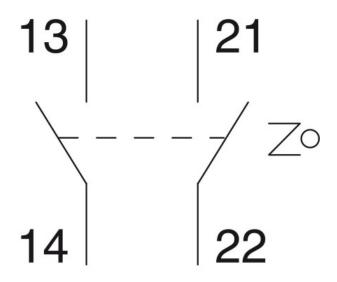
Door contact switch for wall housing - Accessory for cabinet door NSYINLCRN
