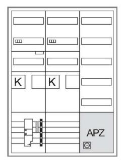
Complete cabinet, univers Z 2 ZP, BKE-I, APZ, VT5 - Equipped meter cabinet IP44 1100x800mm ZB33ET...
