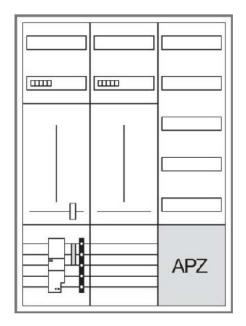
Complete cabinet, univers Z 2 ZP, 3P., APZ, VT5 - Equipped meter cabinet IP44 1100x800mm ZB333T25W31
