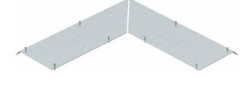
External corner dummy cover On-floor trunking AIKF AEA 25040 Design cover bevelled on one side, with overhang, external corner function, width 250mm, height 37mm, length 800mm, assembly opening without, number of assembly openings 0, material steel, 2-part dummy cover to cover the outer corner of a floor trunking, suitable for trunking bases AIK/U. The sloping cover projects beyond the trunking base at a 45° angle.
