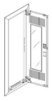
Blind frame with media door for UP-VT, 1x6 rows - Door for cabinet 300mmx950mm steel GBRU16TM
