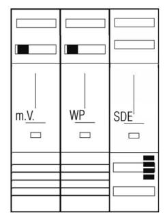
Complete counter space 3pt. 1Z 1WP 1TSG 1V3 o.SH - Meter panel 1 kWh-meters 3 rows Z37E914N
