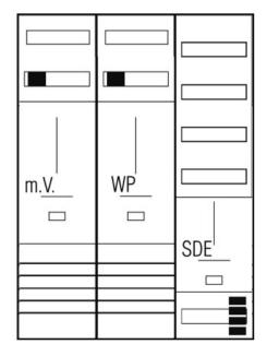
Complete counter space 3pt. 1Z 1WP 1SDE 1V3 o.SH - Meter panel 1 kWh-meters 3 rows Z37D414N
