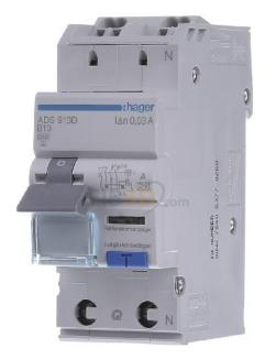
Earth leakage circuit breaker with line protection, two-pole, B-13A 30mA ADS913D
