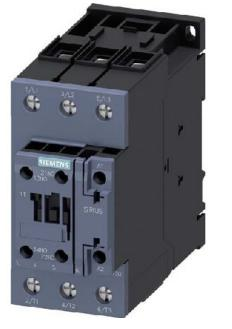
Contactor 18, 5kW/400V, 1NO+1NC - Magnet contactor 41A 175...280VAC 3RT2035-1NP30
